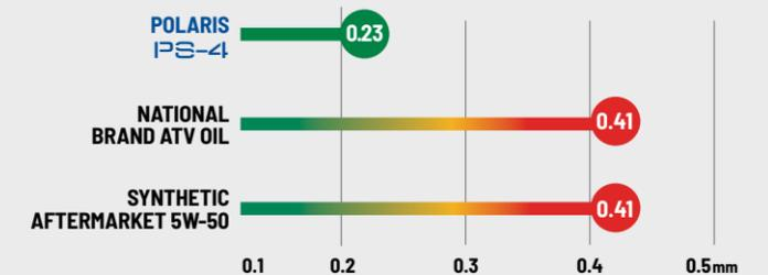
ASTM D4172. In 3rd party testing against 9 competitive products Polaris had 40% or better wear protection compared to all of the tested products. Numbers represent mm of wear scarring measured. Test measures wear at contact points, wear scar is measured for its length and width (in units of mm). Lower wear numbers mean better wear protection and friction reduction.
